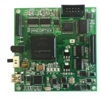
This board has been pre-programmed with HDL code. A VCO nonlinearity correction function embedded on the board can automatically correct the VCO nonlinearity as long as a SDR-RF module has been connected to the board using a FFC cable and a PC is connected by a USB cable.
