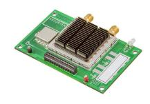
The receiver has an overall 2.8dB low noise figure with two stages of low-noise amplifier and exceptionally linear response with a flat gain of 30dB.
