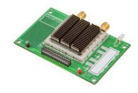
The receiver has an overall 3.4dB low noise figure with two stages of low-noise amplifier and exceptionally linear response with a flat gain of 28dB.
