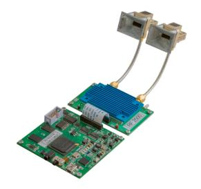
The SDR processor module (SDR-PM 402) is compatible with this SDR-RF 2500B module. The graphic user interface software SDR-GUI is for activating this RF module, selecting operation parameters, and collecting data.
