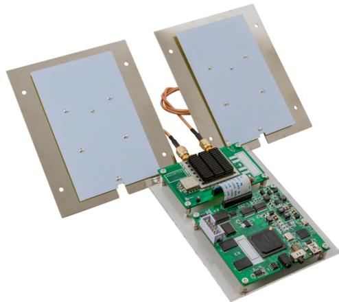
The SDR processor module (SDR-PM 402) is compatible with this SDR-RF 580B module. The graphic user interface software SDR-GUI is for activating this RF module, selecting operation parameters, and collecting data.
