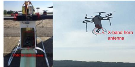
Fig. 1 Drone SAR imaging field test
