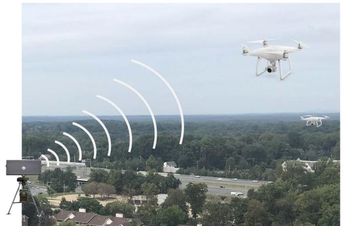
Fig. 1 – Dual-channel Doppler radar tracking drones.
